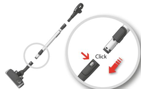
2. **Insert the hose** (to remove it, press the lock buttons and pull the hose out). Insert the hose into the hose handle until the catches click to engage (press the catches to release the hose).
