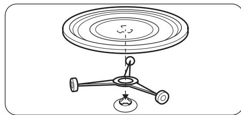
1. Place the roller guide around the turntable shaft.
